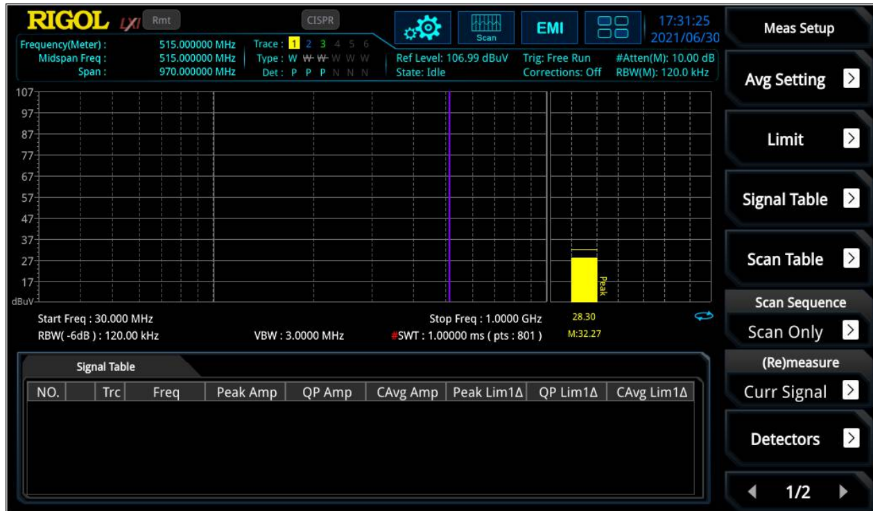
Figure 2: [Meas Setup] Window on right hand side
