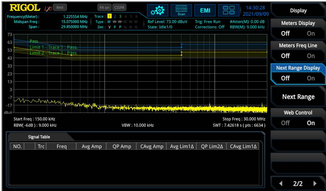
Figure 10: Display modification for bigger trace visibility
