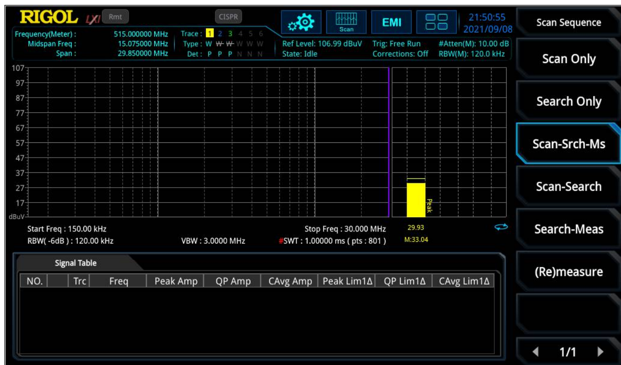
Figure 4: Scan Sequence adjustment with "Scan-Search-Measure"
