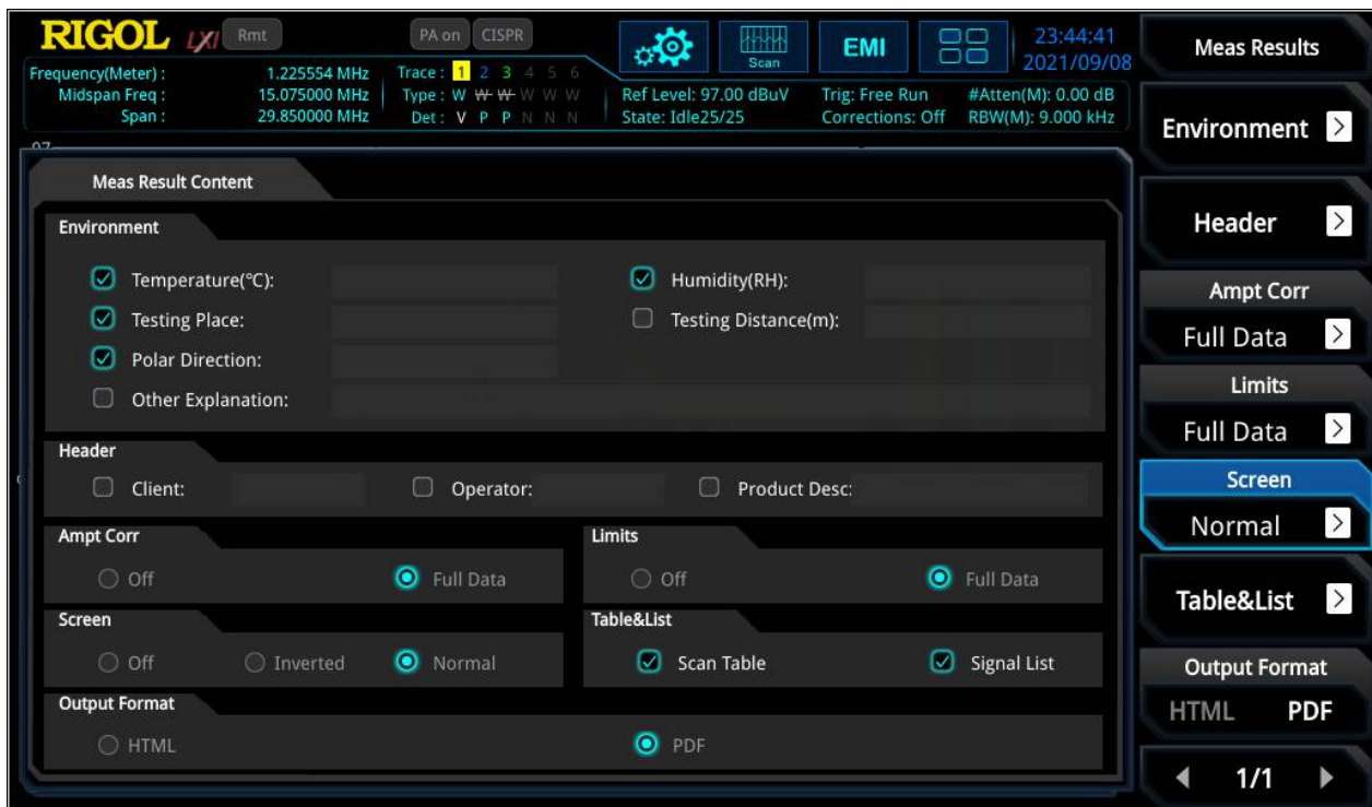
Figure 9: Template to generate a test report for documentation
