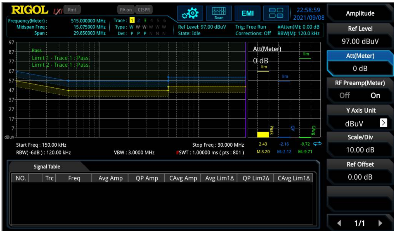
Figure 7: Set dynamic range of measurement meter and the reference level of the test in [AMP]T
