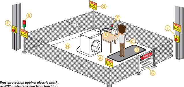
Station without direct protection against electric shock. Such a station does NOT protect the user from touching the DUT during a test.
