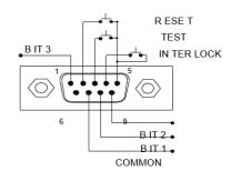
Figure 4.0: SCI Model 4320 Signal Input / Output
