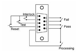
Figure 3.0: SCI Model 295 Remote I/O Connector
