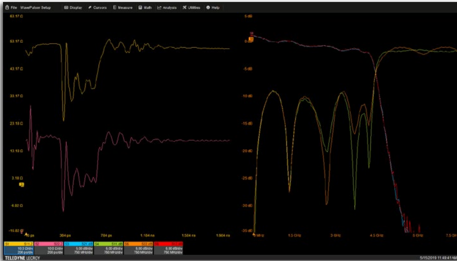
The impedance profile clearly indicates a defective connector in the signal path.
