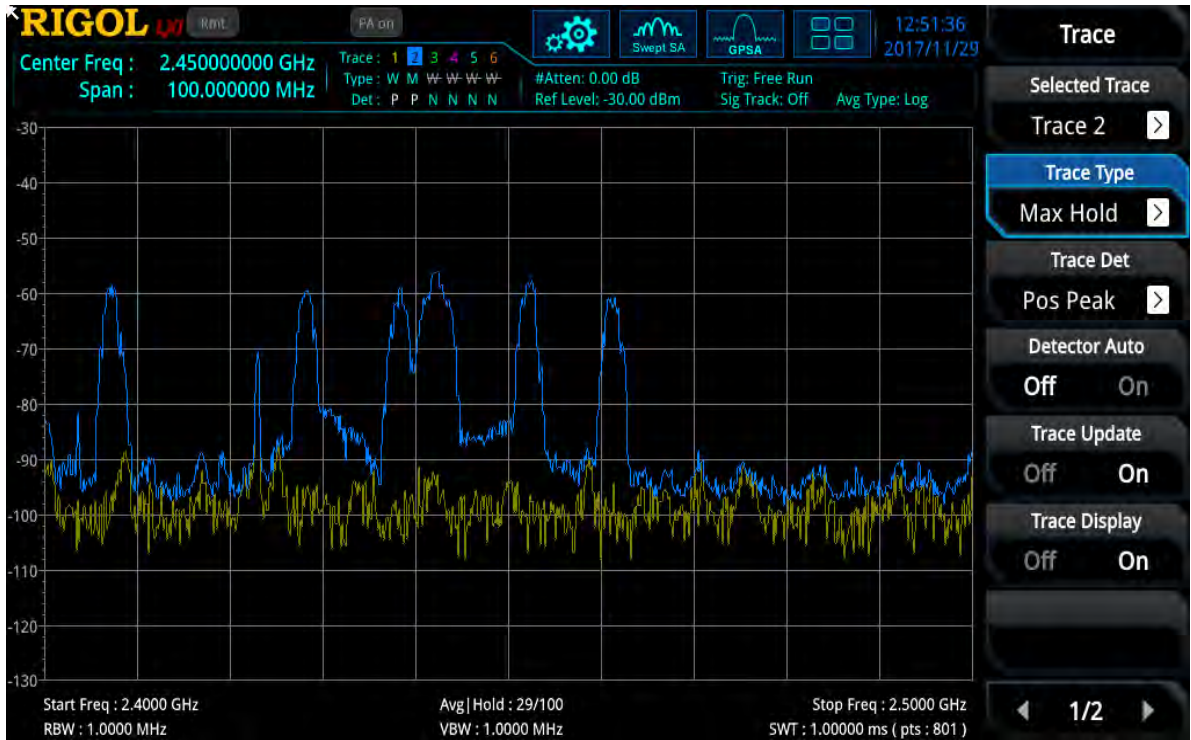
Figure 2: Bluetooth signals are only visible via max hold function with SA
