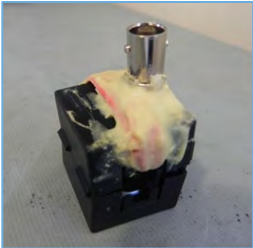
Figure 7-13: Hand-made current probe.
