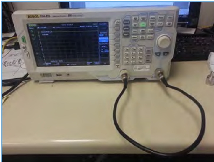
Figure 4-8: Measuring the reference cable.
