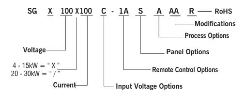
(For units with greater than 3 digits, Voltage/Current is represented in numeric format, e.g., above "100" represents 100A. For units at 1000 and above, the voltage is represented by the format "XKX", e.g, 1K2 = 1200V and 1K0 = 1000V)
