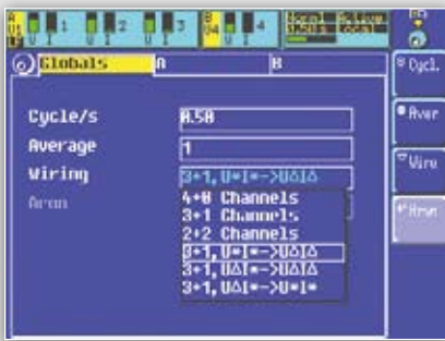
Global settings, shown here is the star-to-delta conversion
