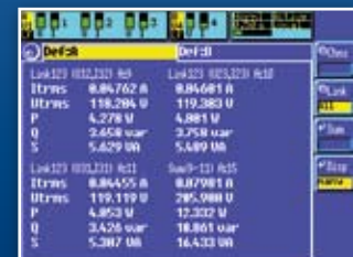
Calculated values (linked values) of the delta-connected windings (wiring: 3+1, U_{\Delta} I^* \rightarrow U_{\Delta} I_{\Delta} )
